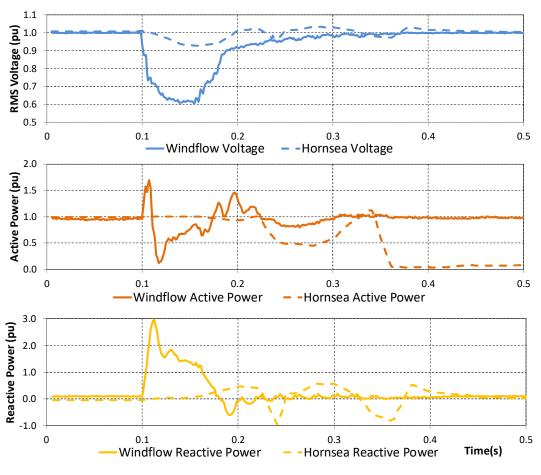
Fig. 2. Comparison of fault response of Windflow 500 synchronous turbine at 48 MW wind farm (8/9/2012) and Hornsea 737 MW wind farm (9/8/2019).
