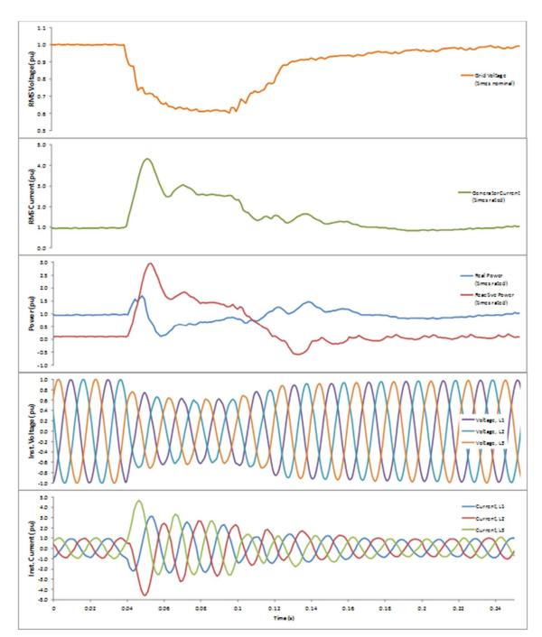
Fig. 1. Fault response of Windflow 500 synchronous turbine during voltage sag event, 8 September 2012, at the 48 MW Te Rere Hau wind farm, New Zealand. This shows an example of short-circuit current contribution and ride-through of a Windflow synchronous turbine during a system voltage disturbance that lasted around 100 ms (0.1 seconds). It is the same basic response as any other "conventional" generating plant on the grid.
