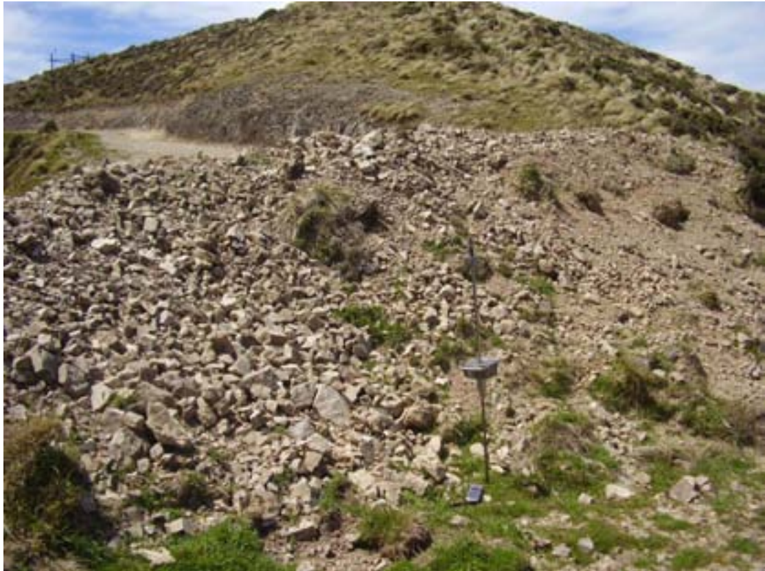
Site 12 – looking north-east with Scala probe in approximate turbine location and 1m-4m high fill batter beyond.
