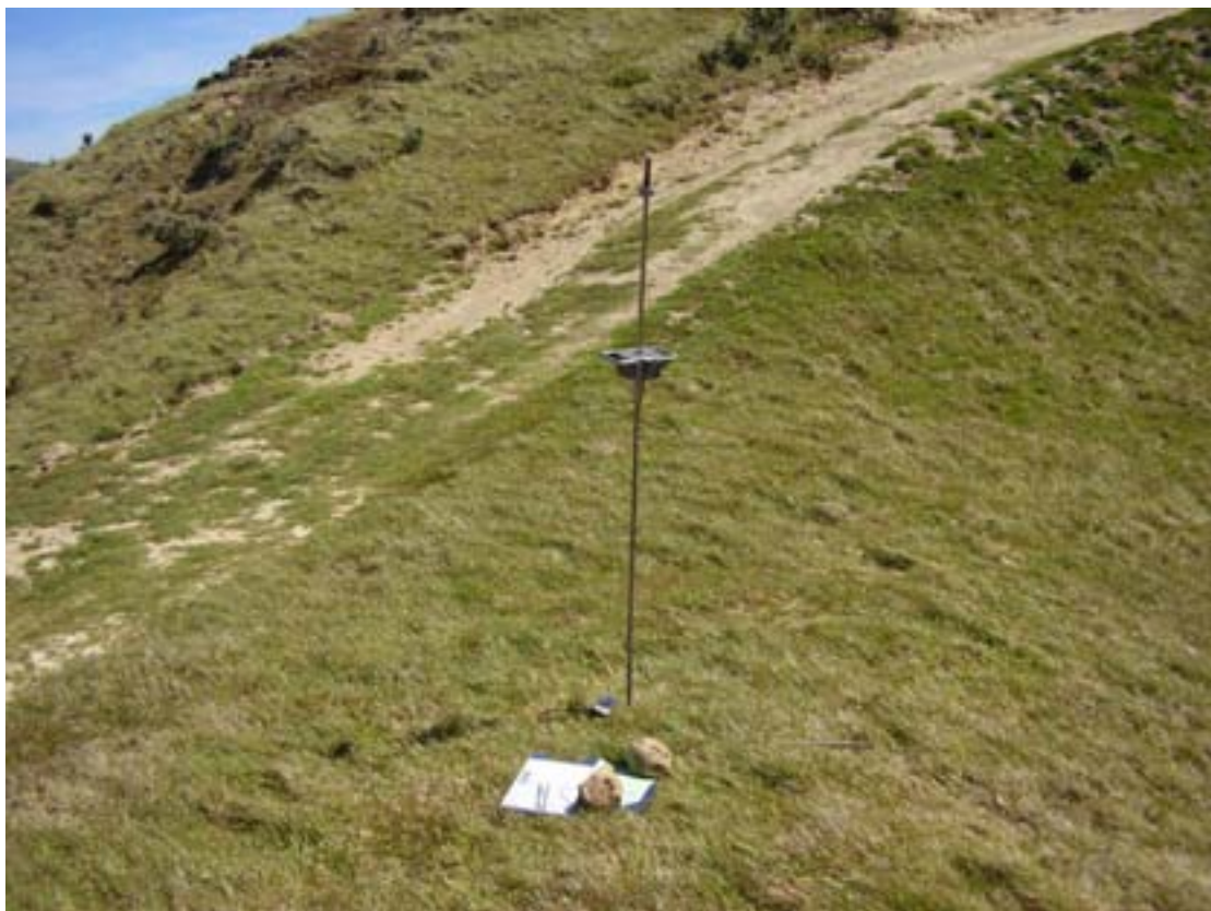
Site 19 – looking south-west with Scala probe in approximate turbine location (location since altered to lie on the other side of the track in the background)
